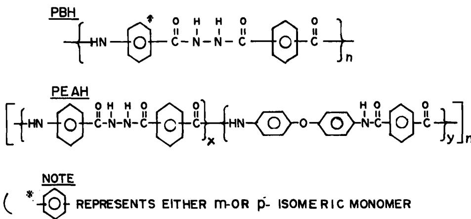
FIG. 1. Possible structures of PBH and PEAH polymers.
